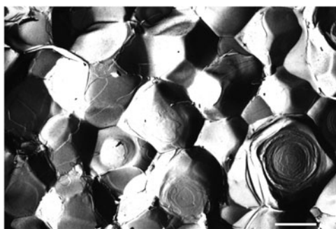
Figure 12. A freeze-fracture electron micrograph of a vesicle phase for a sample of composition 360 mM TDMAO/40 mM TTABr/780 mM 1-hexanol/700 mM NaCl in a H 2 O/glycerol mixture that contains 20 wt% glycerol. The bar represents 2 \mu\text{m} .
